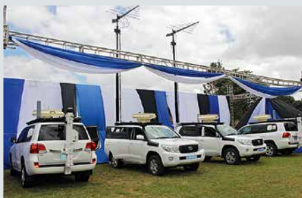
Four off-road vehicles for locating interferers complete the SMMS in Kenya.
