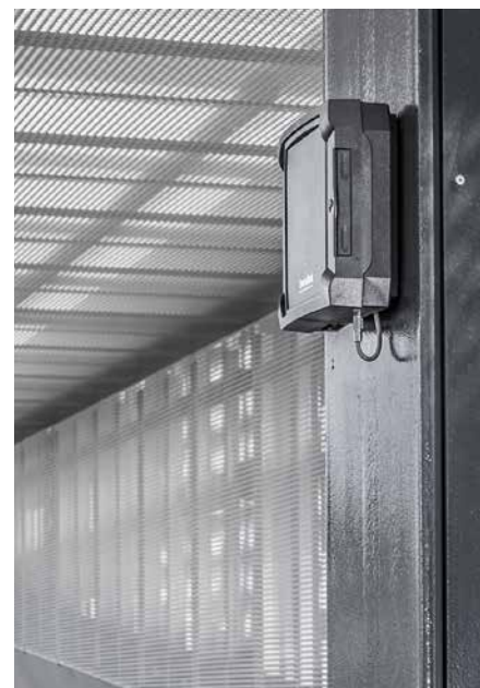
Fig. 3: The compact QualiPoc Remote Control probes from SwissQual can be placed anywhere that mobile networks need to be monitored. Only a power connection is required.
