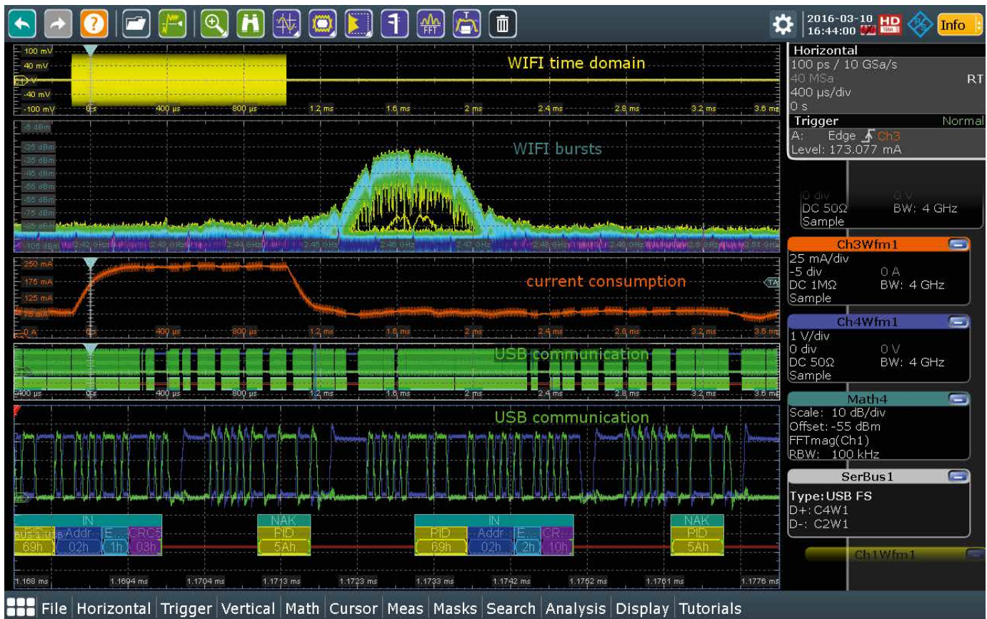
Fig. 3: Example of a multidomain application – IoT module with Wi-Fi radio module, battery-operated power supply and USB interface.
